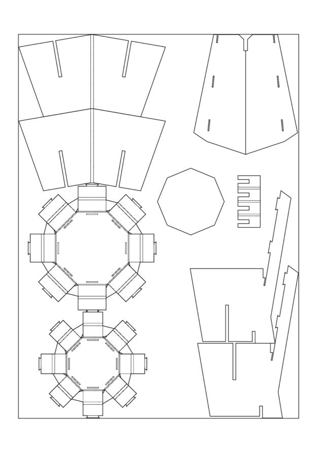
THE OCTA-STOOL COMPRISES OF 9 SEPARATE COMPONENTS THAT USE 60% OF A 1750X2400X6MM SHEET OF DOUBLE WALL CORRUGATED CARDBOARD. THE CUT PLAN SHOWN HERE IS AT 1:12 SCALE.
