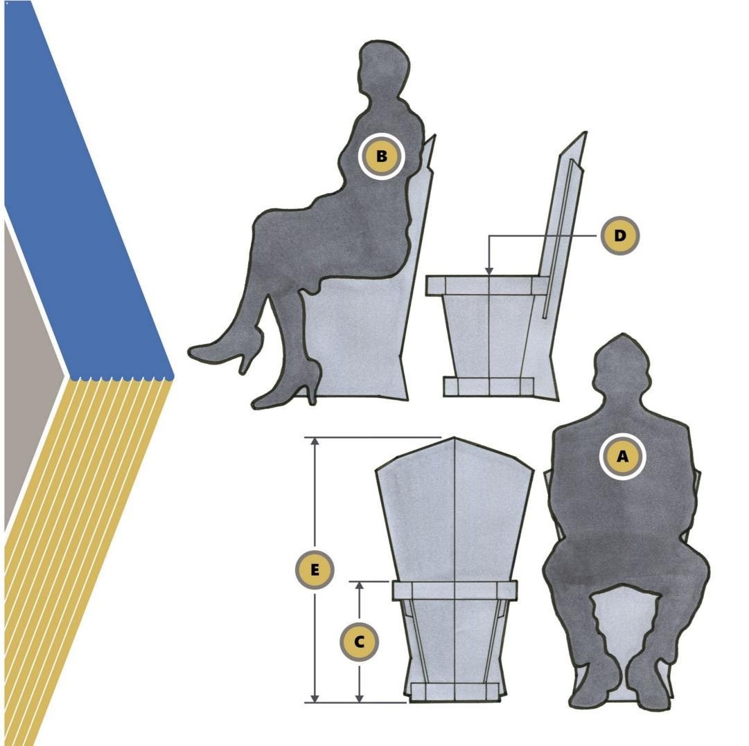
THE OCTA-STOOL WAS DESIGNED AND DIMENSIONED USING MEASUREMENTS TAKEN FROM EXISTING CHAIRS IN ADDITION TO ANTHROPOMETRIC DATA.
